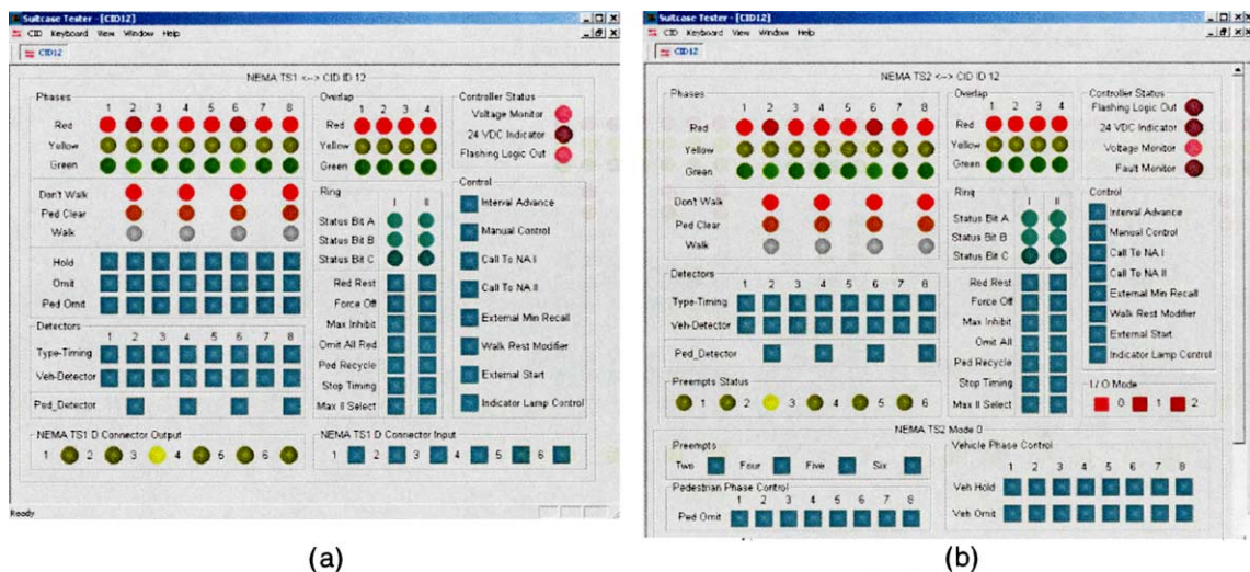
Fig. 6. Example “suit case tester” screens used to setup hardware-in-the-loop simulation: (a) TS 1 display and (b) TS 2 display.
